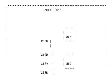
Figure 1 - Location of C140 on Jitter Receiver Module
